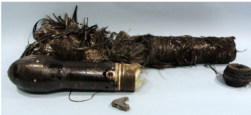
Fig. 13. Scattered parts from one NLAW FM when tested using LPG.
