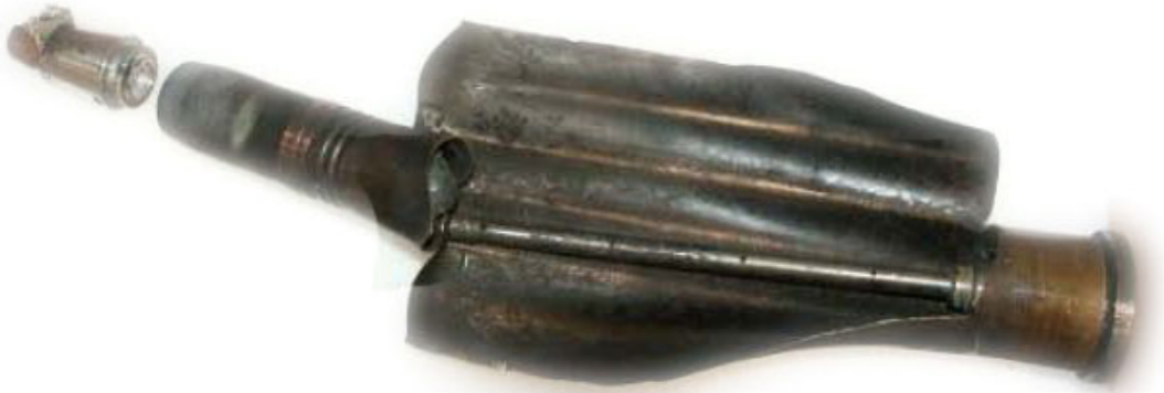
Fig. 8. Scattered parts from one 40 mm L70 LK cartridge case assembly when tested using liquid hydrocarbon fuel.
