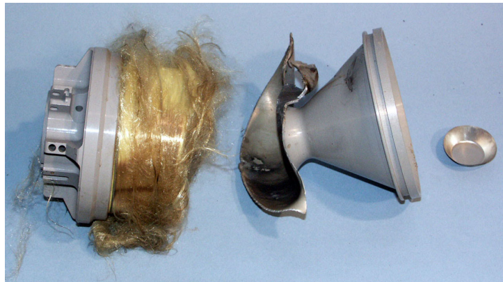
Fig. 11. Scattered parts from one NLAW LR when tested using LPG.
