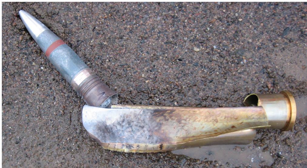
Fig. 9. Scattered parts from one 40 mm L70 LK cartridge case assembly when tested using LPG.
