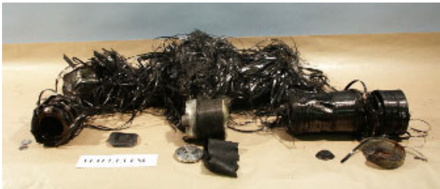
Fig. 12. Scattered parts from one NLAW FM when tested using liquid hydrocarbon fuel.
