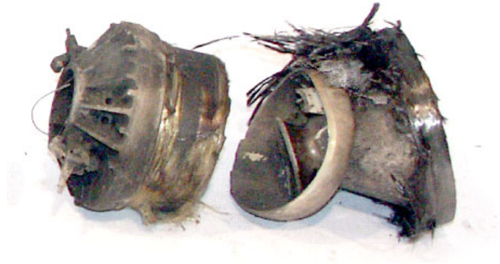
Fig. 10. Scattered parts from one NLAW LR when tested using liquid hydrocarbon fuel.
